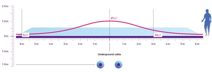
With the cable load factor at a maximum and at a height of one metre, the magnetic field will be no more than 27 microteslas.
